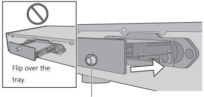
Check the fixing screw position.
