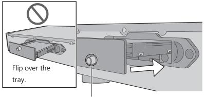
Check the fixing screw position.
