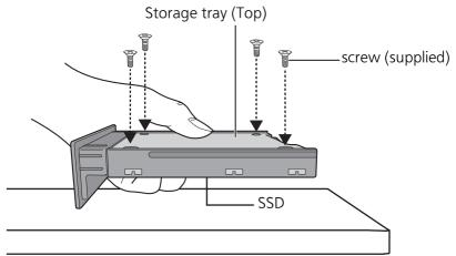
Hold the SSD with one hand to prevent it from falling.
