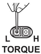
③ After you press the torque button, the confirmation lamp blinks the specified number of times showing the new setting, stays lit for two seconds and then goes off.
