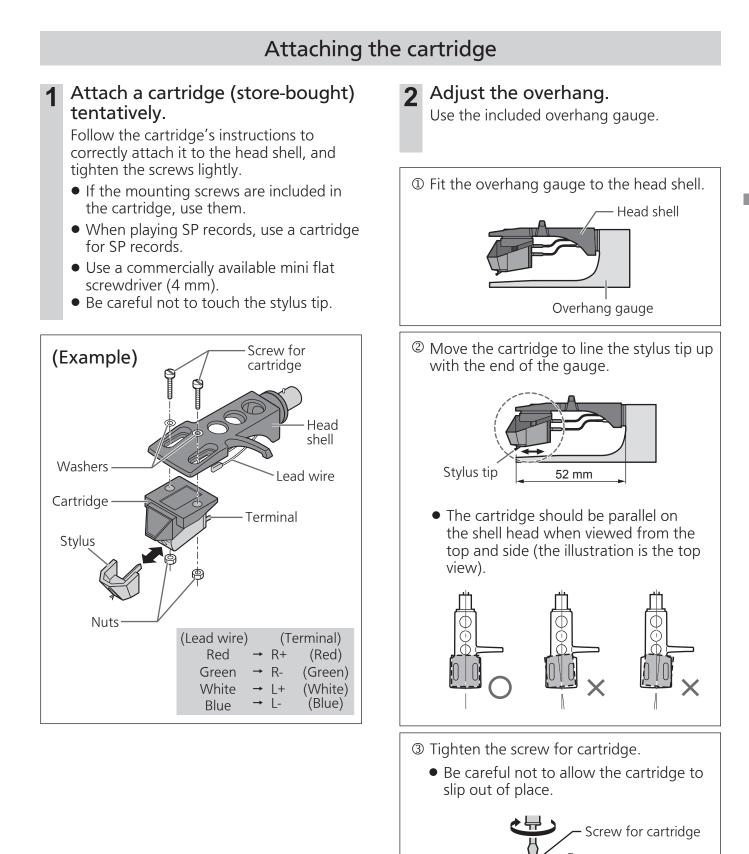
The overhang can be adjusted optimally.
