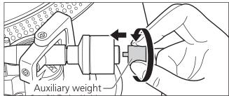
Attach the included auxiliary weight to the rear of the tone arm according to the weight of your cartridge.
