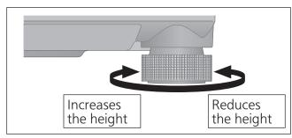
Raise the main unit to turn the insulators and adjust the height.
