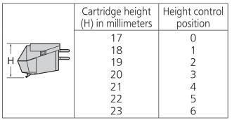
Turn the arm-height control ring to align the position mark with the index line.
